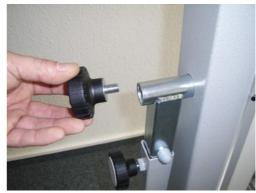
With the fixing screw you can fix the lamp module in the target position.
