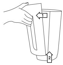
2. Remove the housing cover as shown (magnetic fastening). First detach the magnetic fastening at the top, and then at the bottom.
