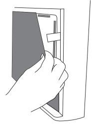
4. Insert a new combi filter. To insert the combi filter correctly, align it with the tabs as shown. Position the pre-filter above it.
