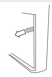
3. Pull out the pre-filter. Now, to pull out the combi filter, pull carefully on the side tabs.
