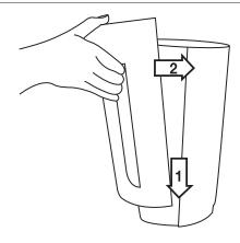
5. Re-insert the housing cover as shown until you see and hear it click into place (magnetic fastening). First attach the magnetic fastening at the bottom, and then at the top.
