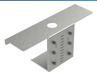
This bracket with a 14-inch-long plate is designed for longer antennas needing a 1.5-inch mounting hole. L bracket includes predrilled holes and slots for mounting. Bottom part of L bracket is solid and allows user to drill holes for customizable mounting.
