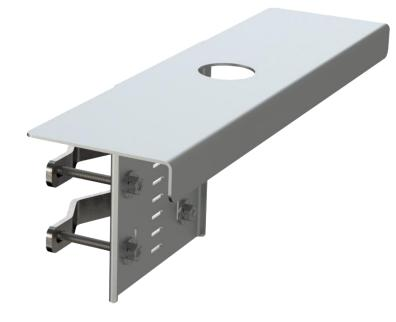
This bracket with a 14-inch-long plate is designed for longer antennas needing a 1.5-inch mounting hole. Bracket is designed to securely fit poles with 1.5 to 2.5-inch diameters or rectangular posts up to 3 inches wide. Additional slots for gear/worm-drive clamps run vertically and horizontally.
