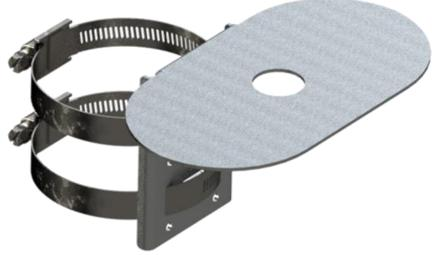
This bracket is designed for smaller antennas needing a 1inch mounting hole. The included adjustable gear/worm-drive clamps fit poles or rectangular posts with 1.5 to 2.5-inch widths. Slots for gear clamps run vertically and horizontally.
