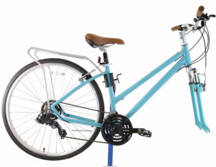
HANDLE BAR / FRAME / REAR WHEEL AND REAR RACK SET-UP seat post is zip-tied to frame
