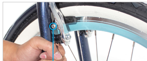
ADJUST WITH 5MM ALLEN KEY
