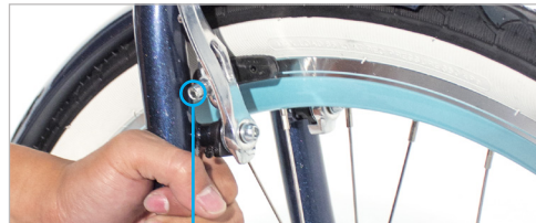
ADJUST WITH 5MM ALLEN KEY
