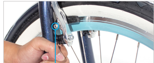
ADJUST WITH 5MM ALLEN KEY
