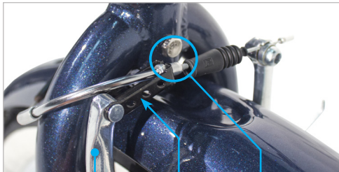
LEFT BRAKE ARM METAL TUBE HANGER END OF METAL TUBE
