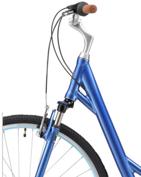
ATTACHED BRAKE CABLE
