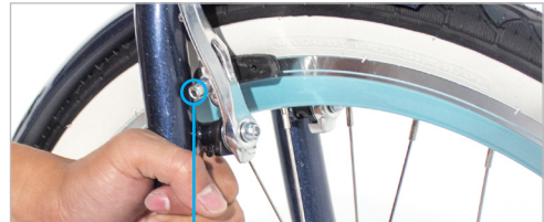
ADJUST WITH 5MM ALLEN KEY
