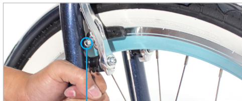
ADJUST WITH 5MM ALLEN KEY
