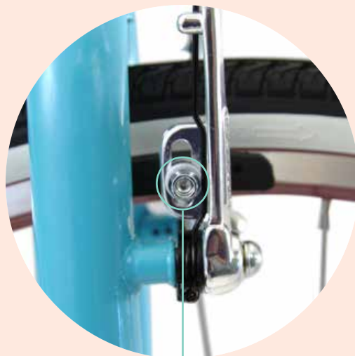
ADJUST WITH 5MM ALLEN KEY
