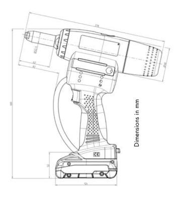
The battery-powered blind rivet setting tool with 20 kN setting force and brushless motor
