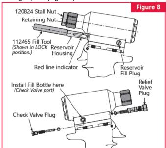
STEP 2: Remove Relief and Check Valve Plugs, Guides, Springs and Balls from ports in head. Reinstall Plug and Sleeve in head in Relief Valve port (front of tool). STEP 3: Screw retaining nut onto Head Assembly. Screw Stall Nut onto Hydraulic Piston and tighten to ensure full thread engagement. Back off Retaining Nut until it engages Stall Nut. Check that Hydraulic Piston is all the way forward and locked with Retaining Nut and with (or without) Stall Nut.
