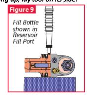
(You may rock the tool to free trapped air in the tool.) Do not allow the air to re-enter the tool. When cycling tool, always hold bottle up as shown in Figure 10 to prevent drawing in air from empty part of bottle.
