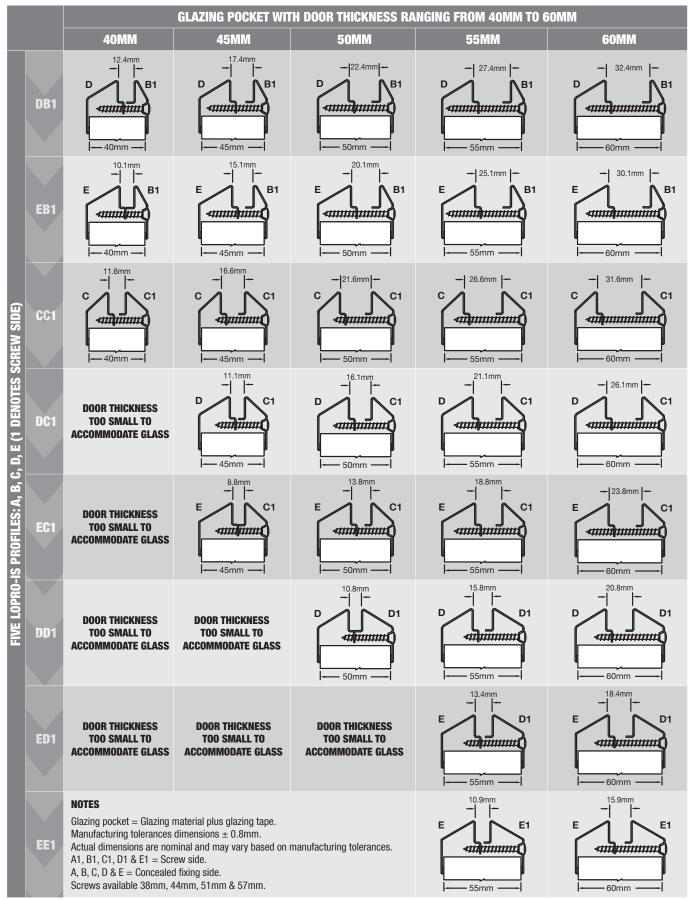
Remember to advise door thickness when ordering to receive correct length screws.
