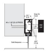
**477AA, 477AA/EC** Sill sweep, snap on cover. Available D & G finishes to order. Optional end caps. (477AA/EC) 477AA 477AA/EC
