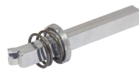
ZSC10 Half spindle. 8 x 8 x 70mm. Zinc plated mild steel. Suits half set of lever furniture. For doors drilled on one side. Suits doors up to 54mm thick. (Box Qty 10)
