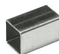
ZSC02 Spindle conversion kit. 8mm to 9mm. Fits in 9mm lock follower so it suits an 8mm lever handle spindle. (Box Qty 10)
