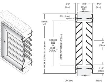
REF SIZE IN INCHES W X H CUT-OUT MM W X H **OUTSIDE FRAME MM** SCREW FIXING STAINLESS STEEL SPLIT Y LOUVRE TO SUIT 29MM MINIMUM THICK DOORS - OTHER SIZES TO SPECIAL ORDER FDLS-SS 0606 6 x 6 152 x 152 196 x 196 **FDLS-SS 0808** 203 x 203 8 x 8 247 x 247 **FDLS-SS 1212** 12 x 12 305 x 305 349 x 349 FDLS-SS 1812 18 x 12 457 x 305 501 x 349 FDLS-SS 1818 18 x 18 457 x 457 501 x 501 **FDLS-SS 1836** 18 x 36 457 x 914 501 x 958 **FDLS-SS 2424** 610 x 610 24 x 24 654 x 654
