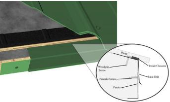
**11. Install eave trim (optional).** Attach eave trim to the lowest purlin on each side. You may use panhead screws (provided by customer) or any screw with a low/flat head that will not interfere with the roofing panels.
