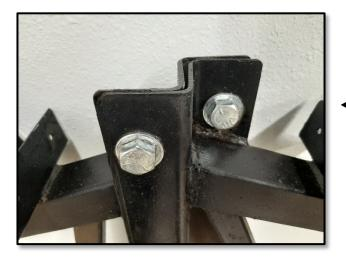
6. Assemble trusses. On the ground, place the two halves of a truss together and secure them with 4 bolts at the truss peak. Use matching nuts and two washers on each bolt (one under the nut, and one under the head of the bolt). Tighten and repeat for each truss as you go.
