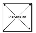
Measure both diagonals of your barn area to ensure the layout is square by finding the hypotenuse of the width and length. (If diagonals are the same, the layout is square).
