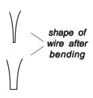
3) Set wire in upper notch of mandrel plate, placing the 'V' or 'U' bend against the side edge of the mandrel plate. Position handcrank as shown and rotate the spring width adjuster in or out so that when the end of the adjuster is against the mandrel plate the distance between the mandrel bushing and the mandrel plate is approximately the width of the spring wire's diameter.
