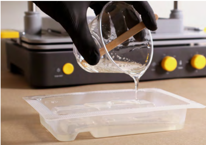
Resin being poured into a Resin Sheet mold.
