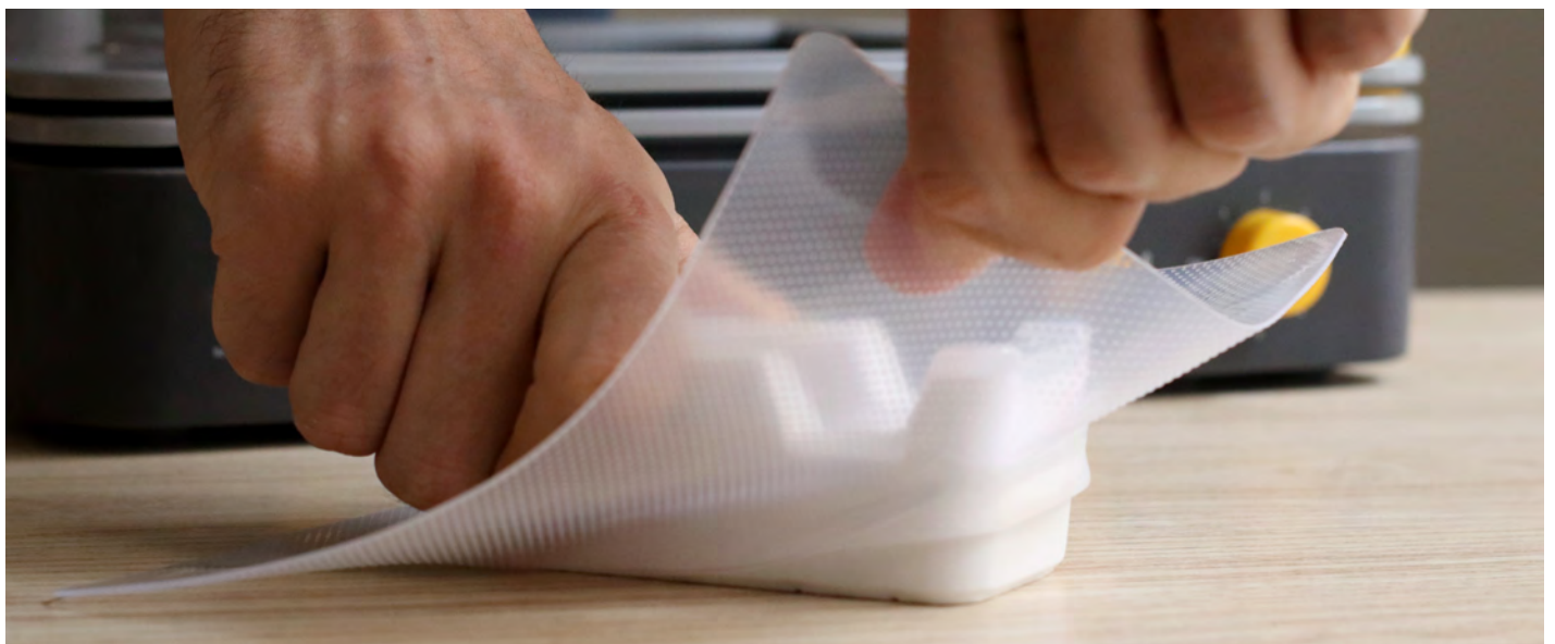
Mold for tape dispenser made on The Mayku FormBox.
