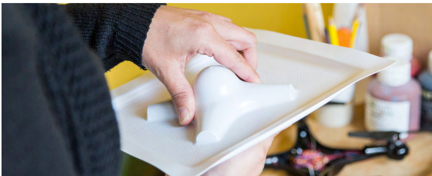
Drone mold made on the Mayku FormBox.
