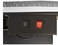
VACUUM, UP-AIR & HEATED SURFACE CONTROLS
