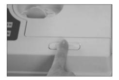
Step 9. When counting is finished, press CLR key to clear the display, The count display will revert to "0".
