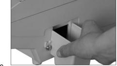
(3) Put the mixed coins into the Hopper and press the START/STOP key to start the counting. After the machine
