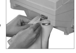
Install the Coin Reject Box onto the side of the machine. If there are a lot of small coins mixed ,
