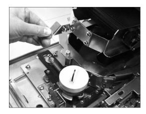
on the conveyor, and at last open conveyor assembly to clear coins in the centrifugal disc. Before the cleaning work was finished, the thickness adjusting assembly cannot be opened.
