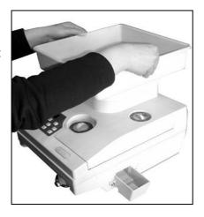
Step 2. Turn on the Power Switch as indicated in the right diagram. The display board will show 0 in the first row and ---- in the second row. The indicating lamp of "ADD" will be on to suggest that the machine is in Accumulation Counting Mode.
