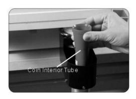
Put the Paper Tube into the Coin interior Tube and the Paper Tube will be held by the Hook Holder
