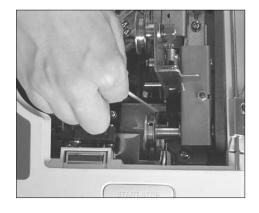
**NOTE:** If small coins with diameter less than 24mm were accidentally put into the capacity hopper with coin quantity adjusting gate is on maximum level, too many small coins will flow into centrifugal disc. The machine cannot be turned on at this time.
