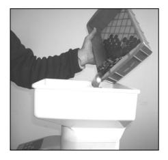
Step 7. Put the coins into the Big Capacity Hopper and press START/STOP key to start counting with quantity displayed on the upper LED line.
