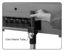
Put the Paper Tube into the Coin interior Tube and the Paper Tube will be held by the Hook Holder
