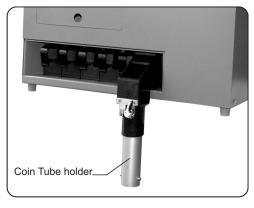
Install the Hook Holder on the Coin Tube Holder.
