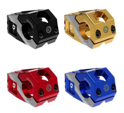
**Hazard:** During our recent quality control inspection, we discovered a manufacturing error that has affected the faceplate of the stem. The faceplate was machined slightly too narrow, resulting in a thinner wall thickness around the four bolt holes. This could potentially cause the
