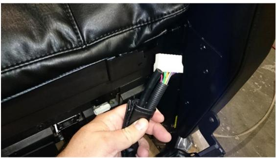
Now plug in the power connector till it clicks in place, and plug in the air hose firmly onto the air nozzle on the chair.
