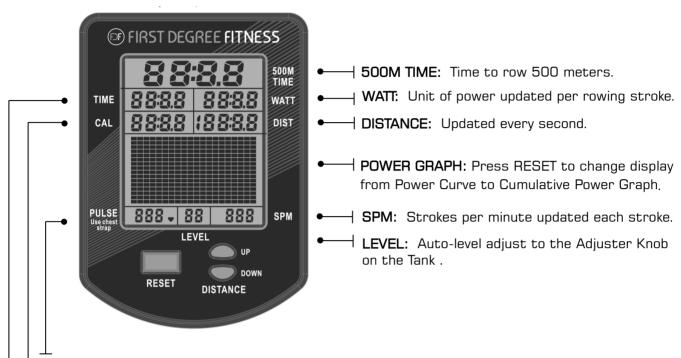
**PULSE:** Updated every two seconds. Compatible with Polar Heart Rate Receiver and Transmitter Chest Strap.
