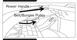
Wind the Rower Belt onto the Belt/Bungee Pulley until the Rower Handle is as it's furthest forward position.
