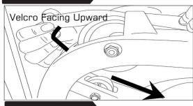
Begin reattaching the Rower Belt by threading around the Rower Belt Pulley with the Velcro side facing upward as illustrated.
