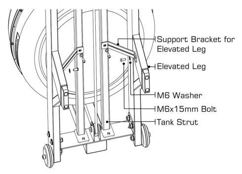
Using 4x M6x15mm Bolt[15], 4x M6 Washer[11], attach the 2x Support Bracket for Elevated Leg[8] to the Rear Brace and Elevated Leg.
