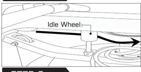
Next, thread the Belt around the Idle Wheel as shown. Once around the Idle Wheel, attach the Rower Belt to the Belt/Bungee Pulley. There is an obvious "lip" at the attachment point.
