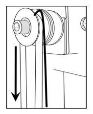
8. Upper left front to lower middle left and right Pulleys.
