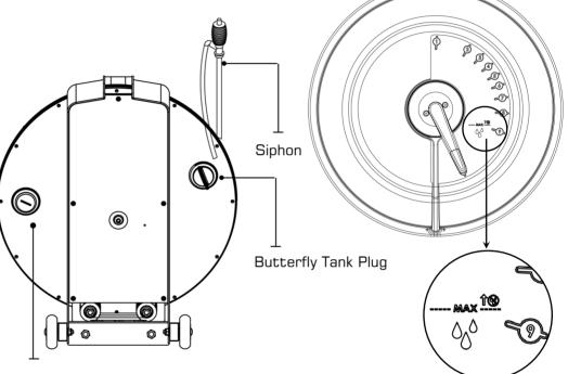
Note: The Lower Tank Plug is permanently sealed
