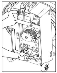
2. Move the Rowing Handle from the S-Bend to a point where it is resting on top of the Tank. This helps line up the Bungee Cord hole for easier removal/replacement. Detach Bungee Cord from lower rear attachment point.
