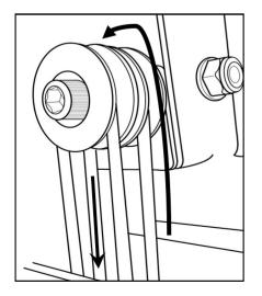
12. Upper left rear Pulley to tie off point. Finish the Bungee rewrap by tying off the Bungee. You may elect to not use a tie wrap as the metal tab is designed as a stand alone attachment point. Thread the Bungee through to desired tension and thread the Bungee end through the upper hole as shown.
