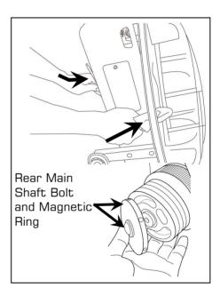
5. After removing the Magnetic Ring and the C-Clip, the Bungee Cord will be accessible. Remove the Belt/Bungee Pulley off the Shaft, pull the Bungee Cord through the Belt/Bungee Pulley and remove. Thread new Bungee Cord through and pull until knotted end is held securely in the slot.
