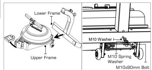
c) Install left and right side Bolts (2x M10x90mm Bolts [14], 2x M10 Washers[18] and 2x M10 Spring Washers [17]). Tighten all three.
