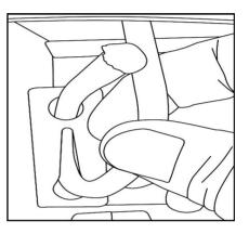
13. Reattach the C-Clip, Magnetic Ring and Rear Main Shaft Bolt. Tighten securely.
