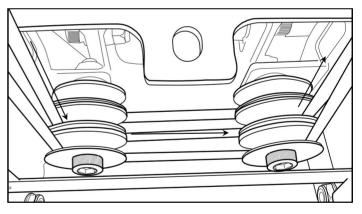
9. Middle right Pulley to upper right Pulley.
