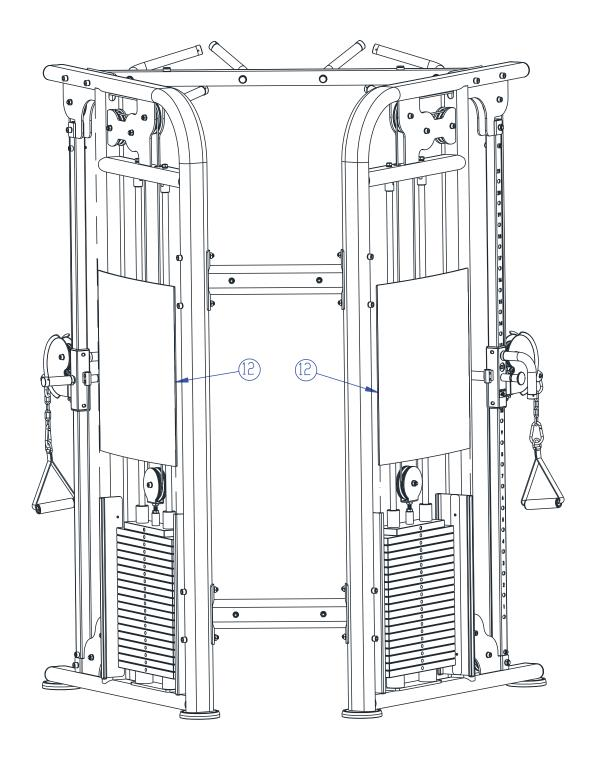
Slide weight stack protective shrouds into the metal grooves on each side of the weight frames with the shrouds bowing out from the back of the selector weight stacks.
