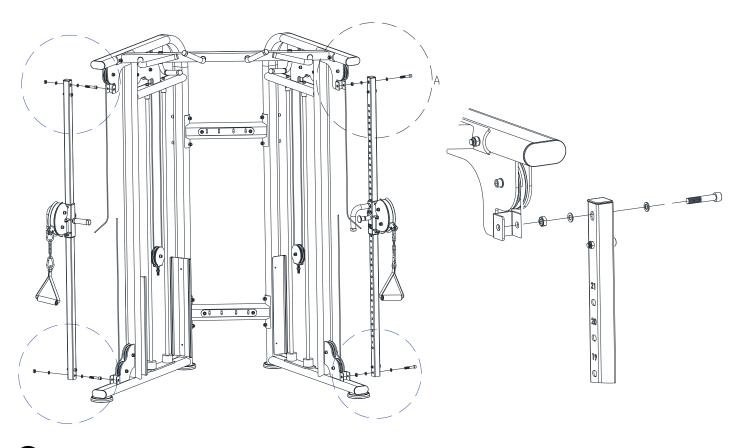
1) Cut the plastic ties that are holding the stainless steel adjustment tubes in place.
