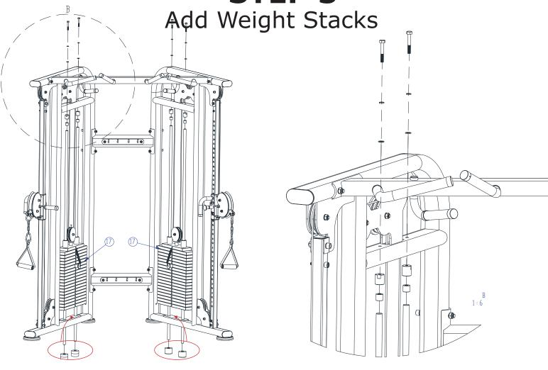
These rubber steppers rest on top of the bottom frame and the weight stacks rest on the rubber.
