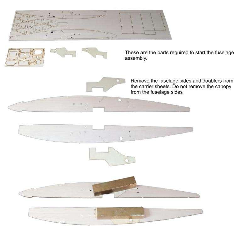
Glue the combined wing dowel and wingeron servo doublers onto the balsa fuselage sides. Make sure you make a correctly handed pair as shown above.
