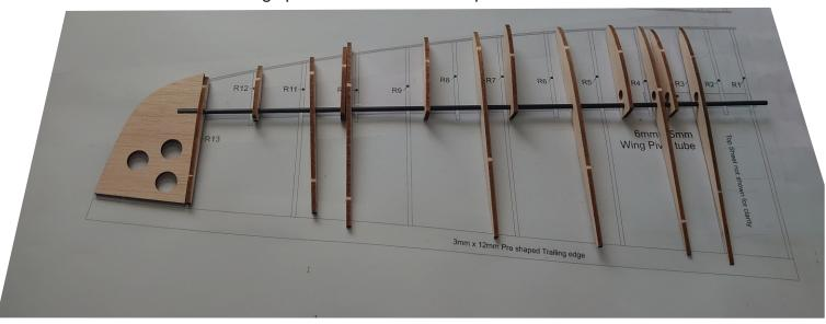
Pin the balsa trailing edge to the plan. The plan must be protected from the glue. You can use a polythene sheet, Clear tape or rub with wax to stop the glue sticking
