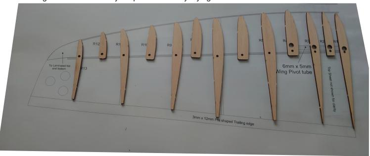
Slide each rib and the wing tip onto the carbon tube spar.
