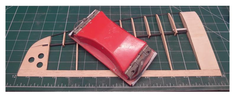
The wing should be sanded using a flat block. We sanded till the slight scorch marks are removed from the ribs.
