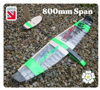
We recommend building your Pug Twisty with "superphatic" adhesive or medium CA. For those of you sensitive to CA fumes we still suggest using it on the carbon to wood joints, so please use an extractor to remove any unwanted fumes, in a ell ventilated room.
