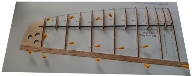
Pin the ribs into place before glueing.
