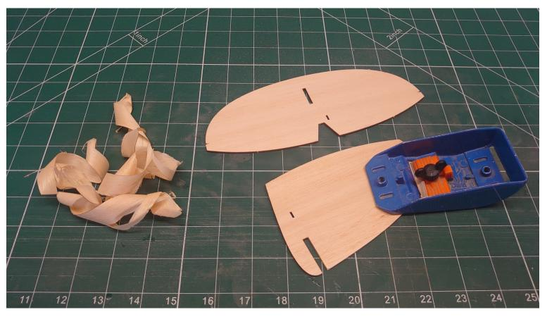
Despite the tail and fin only being 2.5mmthcik we still like to try and carve / sand these to a nice symetrical section. We always aim for a trailing edge thickness of approximatley 0.5mm. This is not critical! If you aren't confident with carving / sanding and covering thin balsa then just a slight taper of the rudder and elevator is sufficient.
