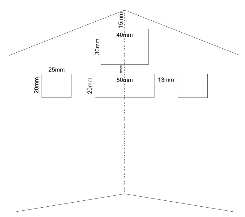
Print this page as a template for cutting the holes for the servos RX and Battery.
