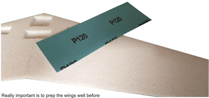
Really important is to prep the wings well before adding the reinforcing tape (not supplied)
