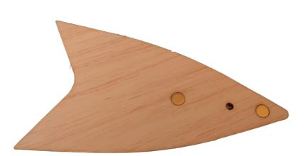
So onto the fins. The fins only need the magnets glueing into place then covering. The magnets that are fitted into the wing have a balsa tip that is basically there just to hold the magnets and give correct alignment. We used hot glue again for this. Make sure you tape over the magnets though. They can pull out if they arent bonded well. Its not a problem though as the smash will fly without one, or both of its fins!
