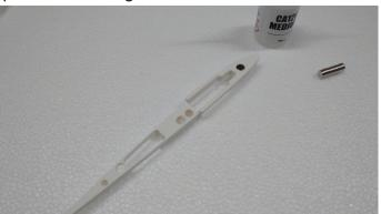
Using Medium CA glue the nose blank onto the left hand root rib. Take care to align this correctly Keeping the magnets in a stack glue one of the 6mm x 1.5mm magnets into the socket as shown
