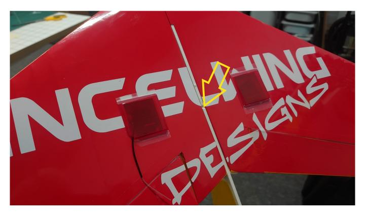
Trim the servo covers with scissors. Ours are painted on the insides before getting taped into place. You can also see we routed one of the antenna out of one of the servo bays. The yellow arrow highlights the C of G point. This is easily identified as an indent on the bottom of the fin keel.
