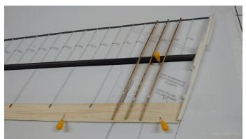
Take care sliding the ribs onto the main spar. They are not a very tight fit but do get more difficult to move around the spar as more of the ribs get glued into place later. The root rib is glued to the balsa TE sheet using medium CA. The balsa ribs are glued to the main spar using the same medium CA. For the balsa to balsa joints we used our TB2 wood glue. Superphatic or regular wood glue can also be used.
