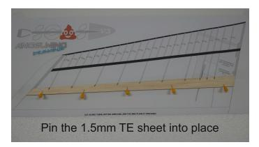
Split the plan so you have a left and right hand wing plan. Our build sequence shows building the left wing first. this isn't critical, just remember to make a left and right hand wing! The plan needs protecting where the 1.5mm balsa trailing edge sheet sits, you can use clear tape or protect the whole plan with a clear polythene sheet if preferred.
