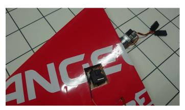
CHA DS06 servo fitted using a very small amount of hot melt glue.
