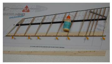
The top trailing edge sheet is glue up against the trailing edge spar, not on top of it. The next image clarifies this
