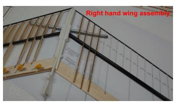
You will notice we do not removed the left hand wing from the plane when we start building the right hand wing. You can if you wish to do so of course. However please note that the right hand wing should always be built, or at least part built with the left wing, and fin keel in place. This ensures you will have a perfectly snug fitting wing join.
