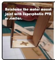
You can of course use some of the scrap 2.5mm balsa sheet to create fillets to strengthen the motor mount joint. We chose not to as we would prefer to knock the motor mount out in the event of a crash than damage the fuselage. "Yes" we have tested the theory.
