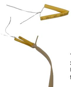
Thread the line through the tubing supplied and tie using 4 knots
