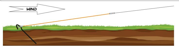
The ground stake must be pushed fully into firm ground at a 45 degree angle away from the wind / launch direction as shown above. The hook of the ground stake should also be pushed into the ground so the rubber cannot be released from the ground stake. Pushing the ground stake in vertically or at the wrong angle could result in the stake being pulled from the ground and fired at speed by the rubber.
