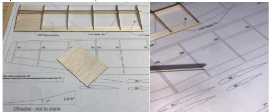
15. Locate one of the center leading edge pieces. This will be easy to spot; it has a notch in one end for the dowel. Glue in place taking care to match the angle of R1.
