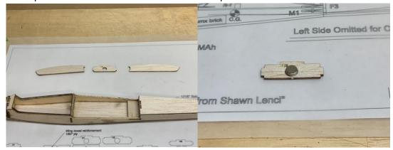
9. Tape the canopy sides and H1 in place on the fuselage. Tack glue H1 to the sides with the smallest drop of CA. *You need to be very careful not to glue the canopy to the fuselage.* Add the top sheeting and tack in place. Remove the canopy and thoroughly glue all the joints from underneath.
