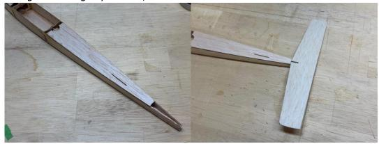
7. Locate the front nose sheeting/hatch. Cuts the tabs and remove the hatch. Dry fit in place, glue when happy. Be careful not to squeeze in the sides, this can make the hatch not fit properly.
