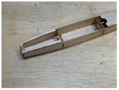
8. Locate the 6 1/8" balsa nose block pieces. Sand the front of F-1 flush and glue on the first (largest) nose block in place. Glue each successively smaller block in place until all 6 are bonded. *Tip:* Use only a drop or two of medium CA and try to keep it in the middle of the block. This will make it easier to sand later.
