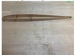
3. Locate the bottom sheeting and fit into place. Once satisfied with the fit it can be bonded. Care must be taken so as to not introduce a warp at this point.
