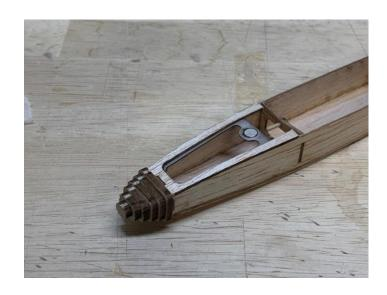
11. Locate the metal washer (in the hardware bag, probably stuck to the magnet ☺) and 1/64<sup>th</sup> ply hatch tongue. Glue the tongue on bottom of the hatch (the side with the etched ring) with the mid line even to the front of the hatch and rounded ends protruding. Using your knife again, remove balsa in the circle so that the washer sits flush with the surface. Glue the washer in place with medium CA. Do not glue in the hatch pull (also on 1/64<sup>th</sup> sheet) at this time.
