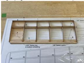
6. Find the 1/32" top sheeting with the etch mark. Taper the sheeting to a point from the etch mark to the edge.
