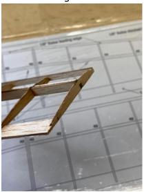
12. Locate the two 1/8" balsa tips and laminate them with medium CA. Take care to get the flat ends as flush as possible.
