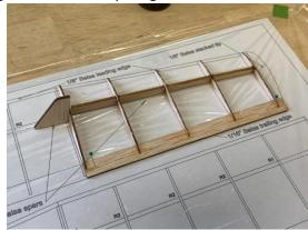
10. Pin the leading edge in place and bond to the ribs. Once dry remove the tip from the plan.
