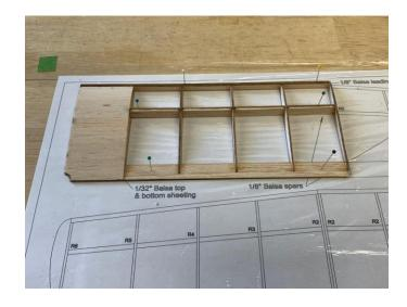
8. Remove the inner wing from the plan and set aside.
