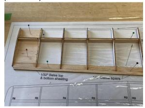
5. Place the 1/8" leading edge up against the ribs and bond in place.
