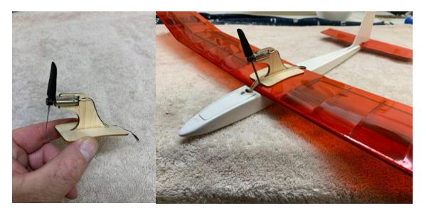
I used an 8mm motor scavenged from a ParkZone Mustang and a Plantraco DD turbo prop. I suspect that there are many other power combos out there that would work equally well or better.
