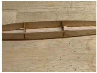
6. Locate the top sheeting and dry fit it into place. Note that the pushrod exit will be on the left side. Bond in place. **Note:** The sheeting does *not* extend all the way forward to F-3. Use the stabilizer to properly locate the sheeting. The aft edge of the stab should overhang the fuselage by about 1/32". **DO NOT GLUE STAB IN PLACE!**
