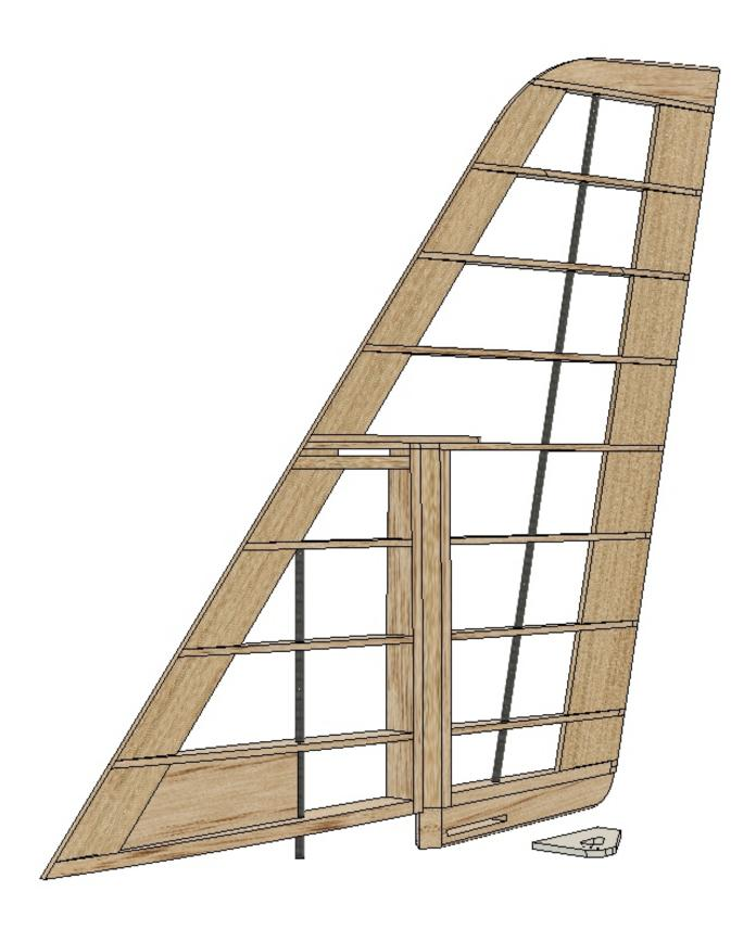
Check the fit of the Rudder horn. Use a needle file to ease the slot if required. Do not glue the horn into place until covering is complete!
