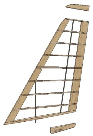
The tip and base of the rudder are made from laminations of 3mm balsa
