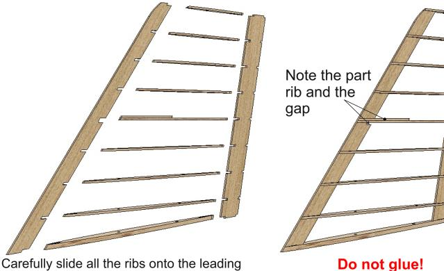
Carefully slide all the ribs onto the leading and trailing edge sheet. Take your time the ribs are cut to nothing and are very delicate at this stage. Do not glue!
