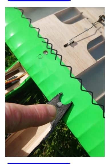
The caopy is retained using a pair of 6mm magnets. One is buried into the canopy itself, the other has been buried into the main center rib. We suggest this is done before covering the model
