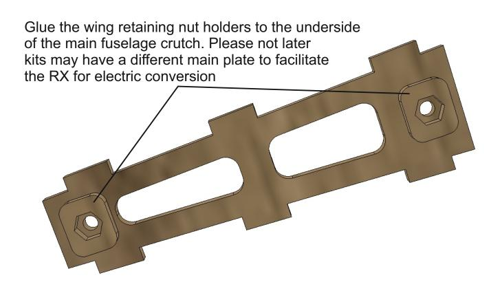
Using epoxy or THICK CA glue the 2 M3 steel nuts into the nut holders. It is essential to keep the threads clear of any adhesive, modeling clay, soft wax etc can all be used to protect the threads from the glue
