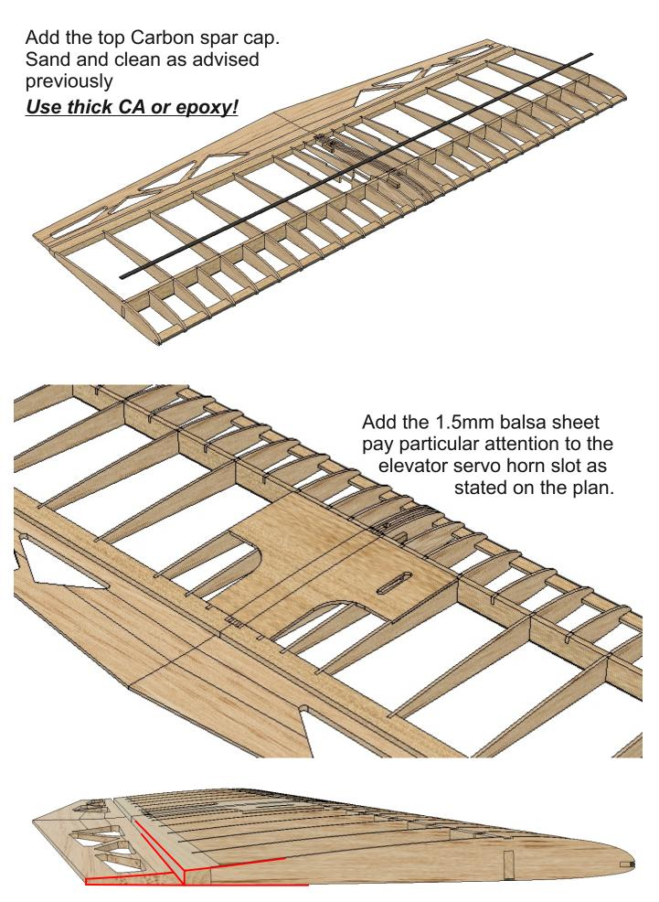
Remove the elevator, with a sharp knife and straight edge Add a chamfer to facilitate **bottom hinging!**
