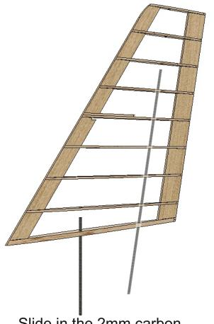
Slide in the 2mm carbon tube spars, slowly twisting helps, as done sanding a slight point to the top of the spars
