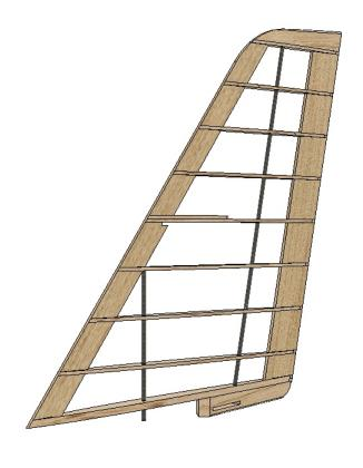
At this stage the assembly can be sanded if prefered. Just a slight radius on the leading edge is required and the tip and base blocks sanded to match the rib profiles and rounded
