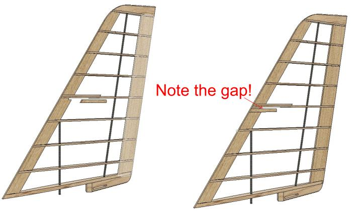
Pin into place the 3mm rib that forms the top of the fin. This can be adjusted later when the Leading and trailing edges are added
