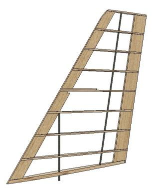
Once the spars are in position with the fin assembly held accurately over the plan you can now glue the assembly together. Use CA for carbon to balsa. We suggest either superphatic or laser cut wood glue for the wood to wood joints
