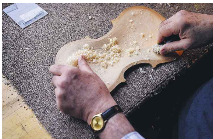
Rufino uses a tiny thumb plane to carefully hollow out a side of a violin he is building.
