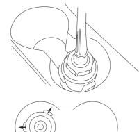
Expand the base arms by turning the base expansion knob clockwise. Then bend and make adjustments to the gooseneck as needed.
