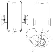
To utilize the side cable management hanger, simply pull it downward and place your charging cable into the hanger.
