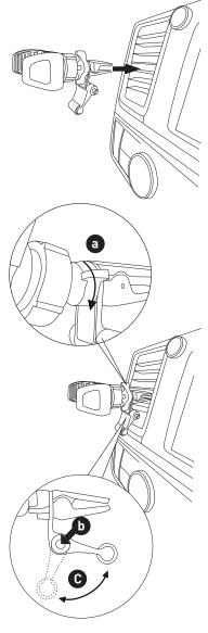
3. Once the clamp is securely in place you can loosen the ball-joint to rotate and angle the clip holder toward driver, and turn to tighten the ball-joint. Then simply press-in on the clip lever to open the clip holder and place your phone inside.
