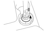
3. Slide the tray onto the top tray slot opening then loosen the tray and arm angle adjustment screws to make adjustments to the tray as needed.
