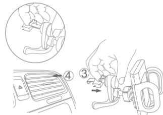
9. Slightly unscrew the ball-head cap clockwise to loosen up the ball-head and adjust the viewing angle of your device with tilt and 360 degree rotation of the cradle.
