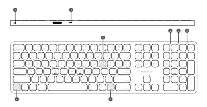
The first time using with a Bluetooth device, pairing is needed. Press Fn and P keys simultaneously, the pairing LED will blink indicating the keyboard is in pairing mode.
