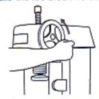
4) Turn the Lock knob clockwise and lock the main shaft.
