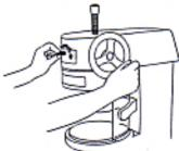
By holding the upper end of main shaft, turn the ice block holder at the other end of the shaft counter-clockwise and remove it from the main shaft.
