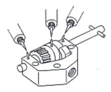
3) Use gear oil for oiling. Other mineral oil, such as machine oil can also be used.
