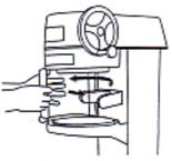
Remove wing bolts (2pcs) fastening shaving plate at back of the plate. Raise the shaving plate and remove it.
