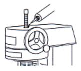
For oiling the crank, remove head cover and oil through the two small oiling holes located on the upper part of the bearing.
