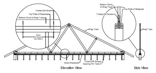
Figure 2: Drag Strut Truss Connection to Shear Walls
