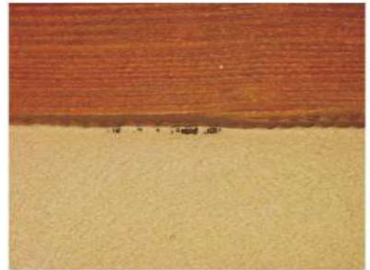
Small repairable tear
