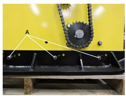
The drive chain may loosen over time and need to be adjusted. This is done by removing the motor
