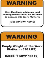
One each on the back of each MWP 4x116 Work Platform
