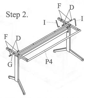
STEP 2: Attach flip top release mechanism to legs with (F), (D), and (G).
