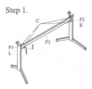
STEP 1: Attach left and right legs to middle support with (4) C hex bolts
