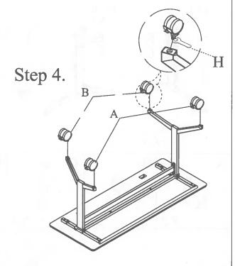
STEP 4: Attach (4) casters to feet and tighten.
