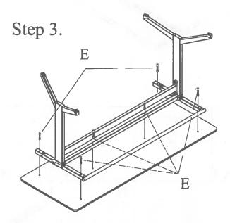
STEP 3: Attach top to base with (6) E Screws
