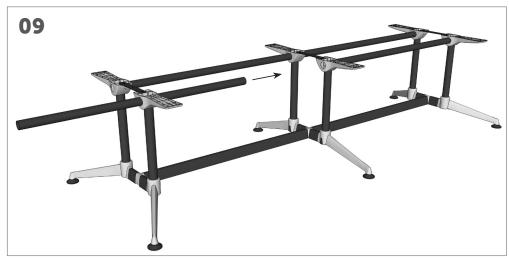
Slide each top rail through the upper wrists, making sure they are located in the centre of the frame.
