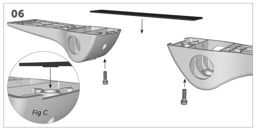
Place the steel strap onto the upper wrists, with the raised areas of the straps slotting into the holes on the upper wrist, *Fig C*. Fully tighten the M8x25mm bolts. (*Repeat with all upper wrists and steel straps*)
