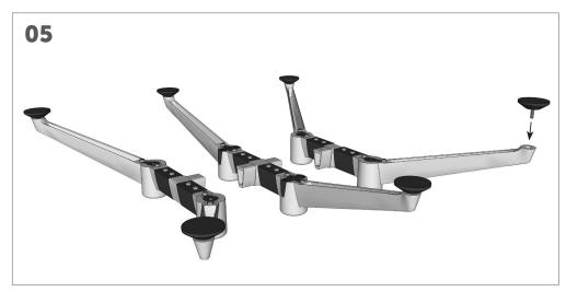
Screw all glides into the base of the large feet, leaving the glides one turn from tight (then they can be adjusted easily if the floor is uneven).
