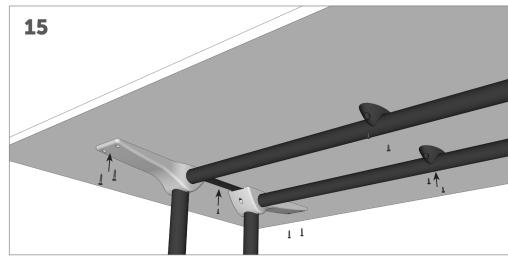
Fully tighten all M5x30mm screws through each upper wrist into the work surface. Fully tighten all M5x20mm screws through each steel strap and plastic support into the work surface.
