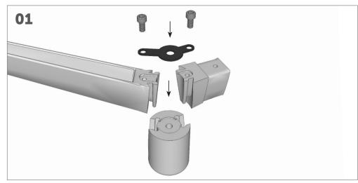
Slide the large foot and T tube connector into the collar, place the 150° gasket on top, and fully tighten the 2 M8x16mm bolts into the collar. (*Repeat with all 150° collars*)
