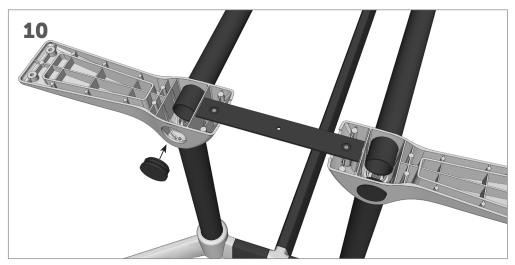
Place the top rail caps into the exposed holes on each end of the frame assembly.
