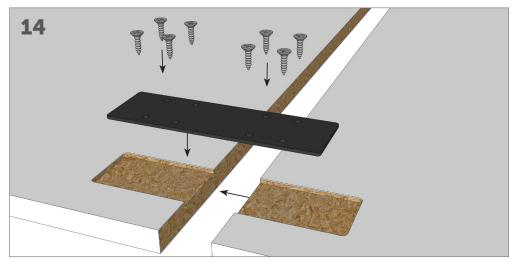
For multi piece work surfaces, use the table top bracket plates, and M5x20mm screws to join together as one solid piece. This should be done with the work surface sitting on the frame in its final position.
