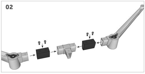
Using 2 T tubes, connect the assembled corner feet to the bottom T connector, and fully tighten the 4 M8x16mm bolts. (Repeat with all 150° feet)
