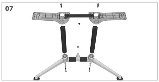
Place a feet tube on top of each collar, and the upper wrist assembly on top of the feet tubes. Fully tighten the M10x30mm bolts through the upper wrists, and M10x110mm bolt, spring washer and flat washer through the collars.
