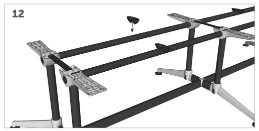
Snap the plastic support brackets onto the centre of each top rail. The frame assembly is now complete.
