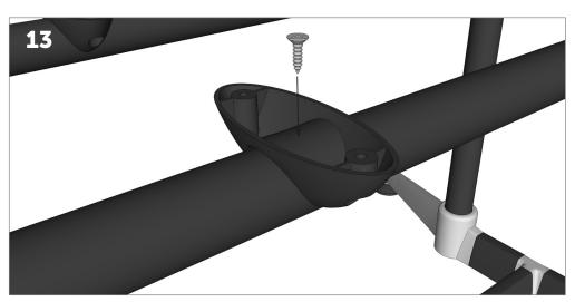
**Optional**: For extra strength, the plastic support brackets can be screwed onto the top rails.
