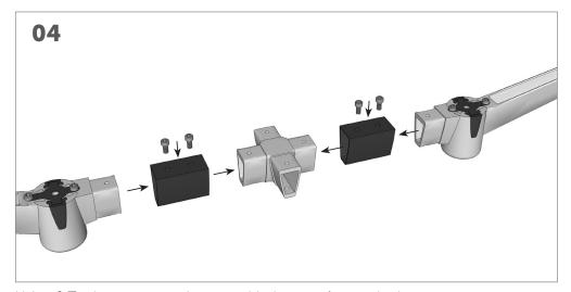
Using 2 T tubes, connect the assembled centre feet to the bottom cross connector, and fully tighten the 4 M8x16mm bolts.
