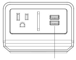
3.1 amp USB quick charging module can charge one tablet and one smart phone at the same time.
