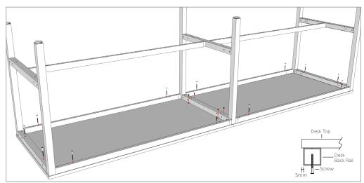
**COMPLETE:** Pre-drill holes into the worktop, place worktop on a clean, flat surface and fully tighten the worktop to each rail using the provided screws. Using 2 people rotate table into upright position.
