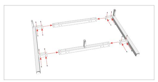
**STEP 1:** Assemble corner legs and short rails together and fully tighten with provided screws.
